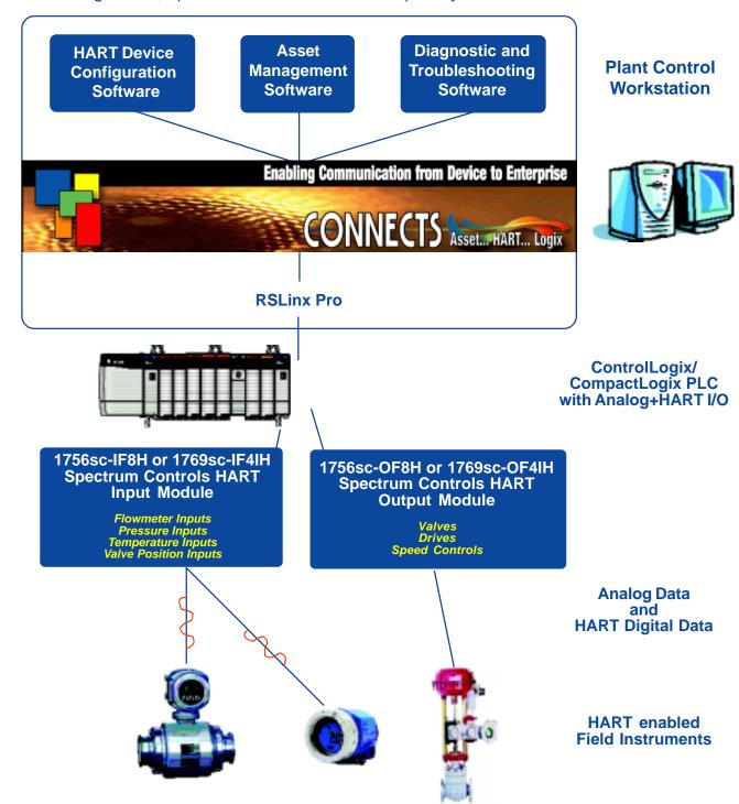
A CompactLogix PLC can be the HART gateway for a complete plant control system. Asset management, system configuration and maintenance tasks that required personnel to acquire data from the factory floor can now be easily performed from a single workstation or enterprise network.
