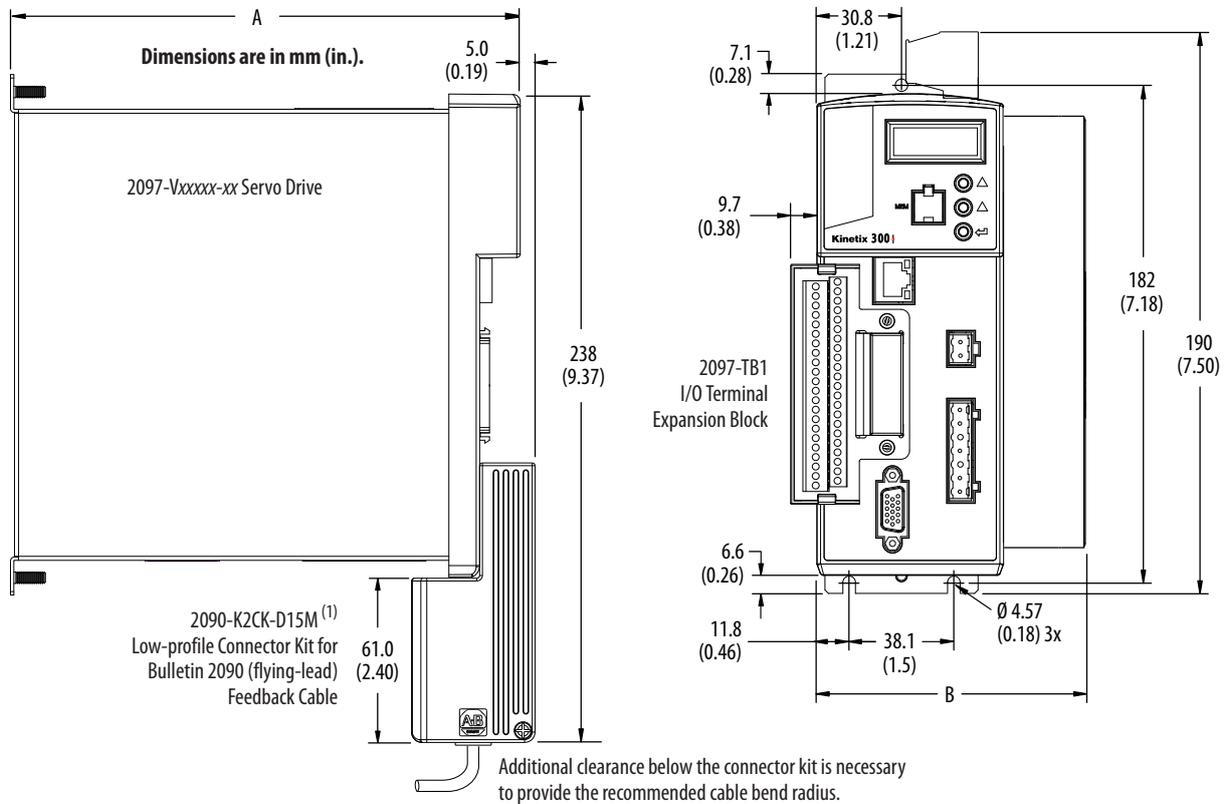
(1) Use the LDAT-CONKIT-ABS connector kit with added circuitry for Kinetix 300 drives and LDAT-Series linear thrusters with absolute high-resolution encoders. Both kits have the same physical dimensions.
