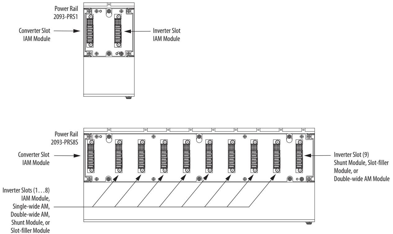
For example, the 2093-PRS1 power rail contains one inverter slot. This limits the use of this power rail to systems requiring only one inverter slot. Similarly, the 2093-PRS2 power rail contains two inverter slots. This limits the use of this power rail to systems requiring up to two inverter slots. When selecting a power rail, determine the number of inverter slots required by all rail-mounted modules and select one with that minimum number of inverter slots.
