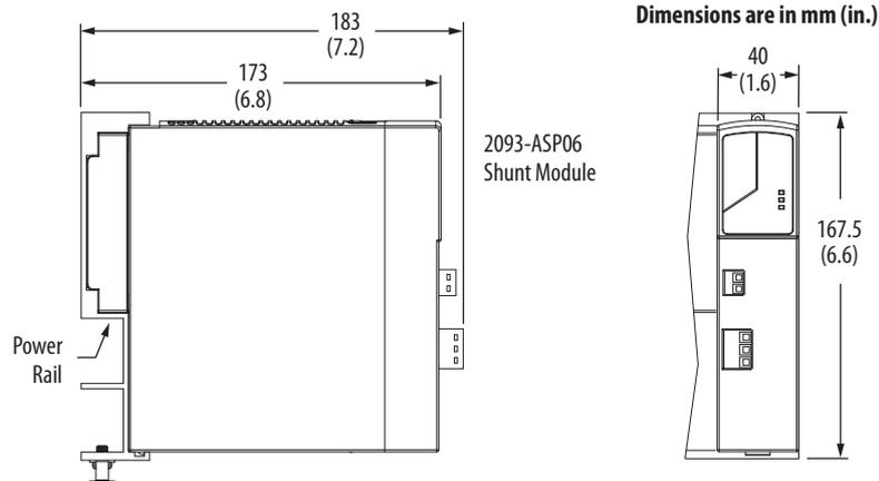
Modules are shown mounted to the power rail and the dimensions reflect that.
