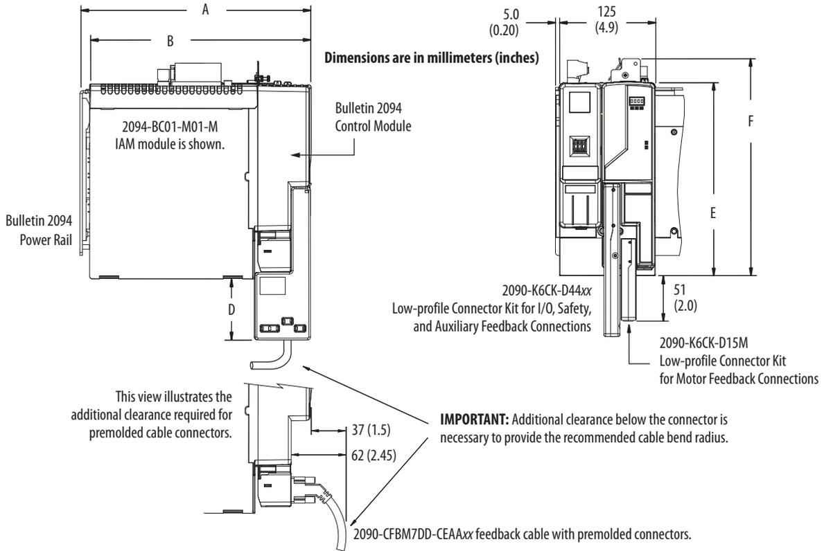
The IAM power module is shown mounted to the power rail with the control module attached.
