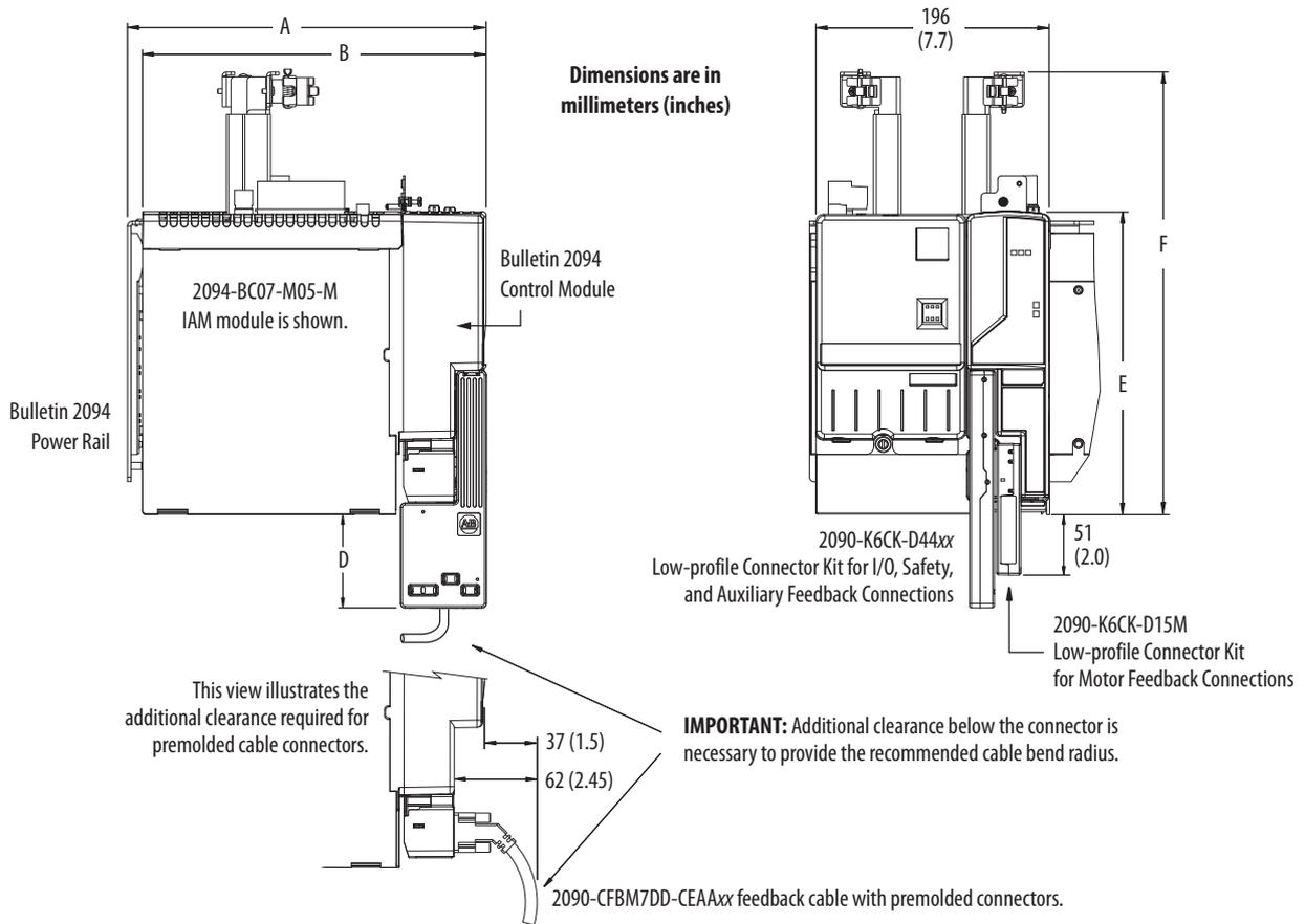
The IAM power module is shown mounted to the power rail with the control module attached.
