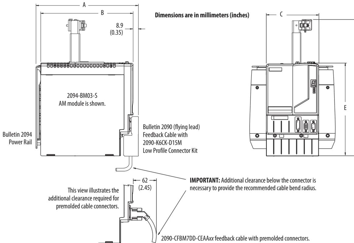
Modules are shown mounted to the power rail and the dimensions reflect that in the depth of the module.
