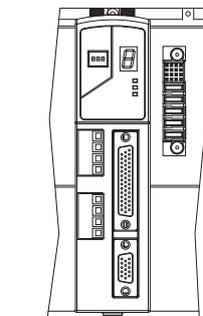
**IMPORTANT:** Additional clearance below the connector is necessary to provide the recommended cable bend radius.
