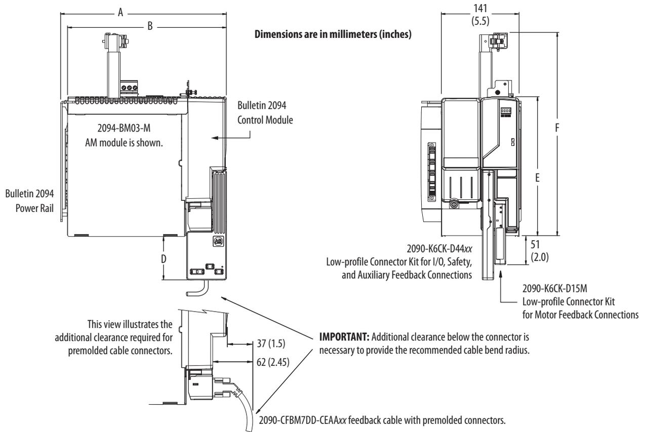
The AM power module is shown mounted to the power rail with the control module attached.
