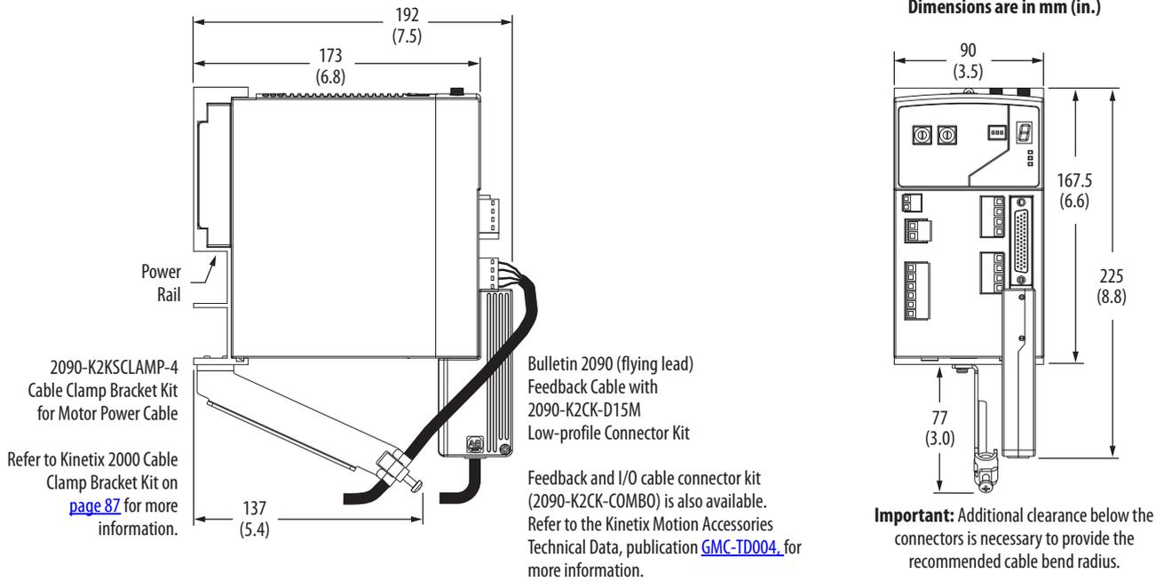
Modules are shown mounted to the power rail and the dimensions reflect that in the depth of the module.
