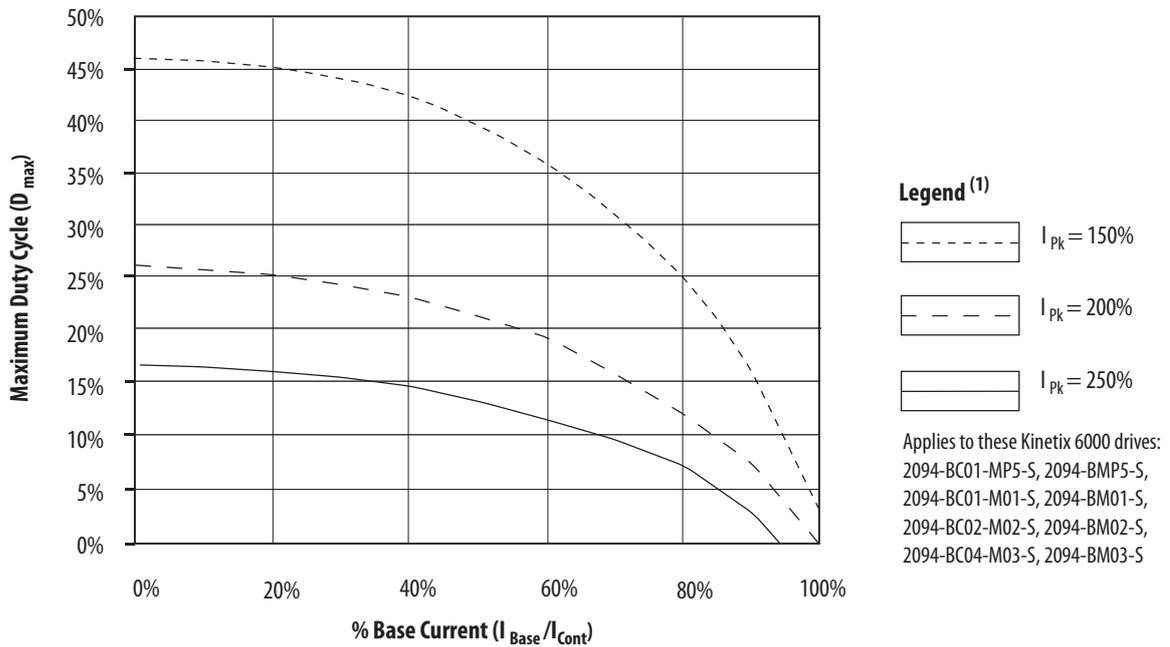
(1) Base current ( $I_{Base}$ ) and peak current ( $I_{PK}$ ) are a percentage of the continuous drive current rating ( $I_{Cont}$ ).
