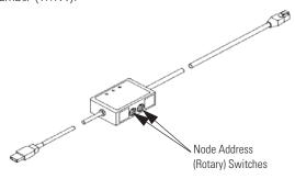
2. Insert the end of the cable having the USB connector into a USB port on a computer.
